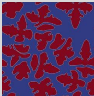
Multigrain simulation of AlZn alloy using OpenFOAMsolver.
